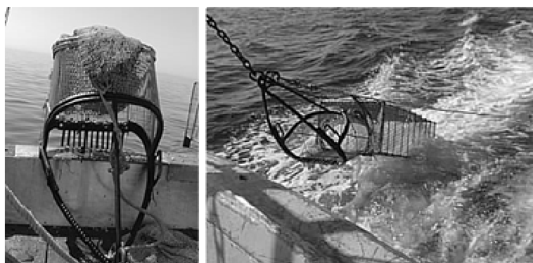
Figure 6. Traditional dredge (TD) and grid dredge (GD).
