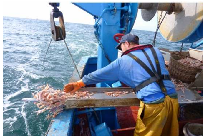
Figure 11. Sorting gutter to discard the commercial catch all along the sorting process on board.
