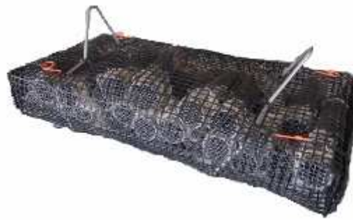
Figure 2b. Re-immersion bag containing 25 plastic tubes.
