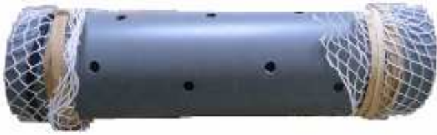
Perforated plastic tubes for re-immersion of individual discarded Nephrops
